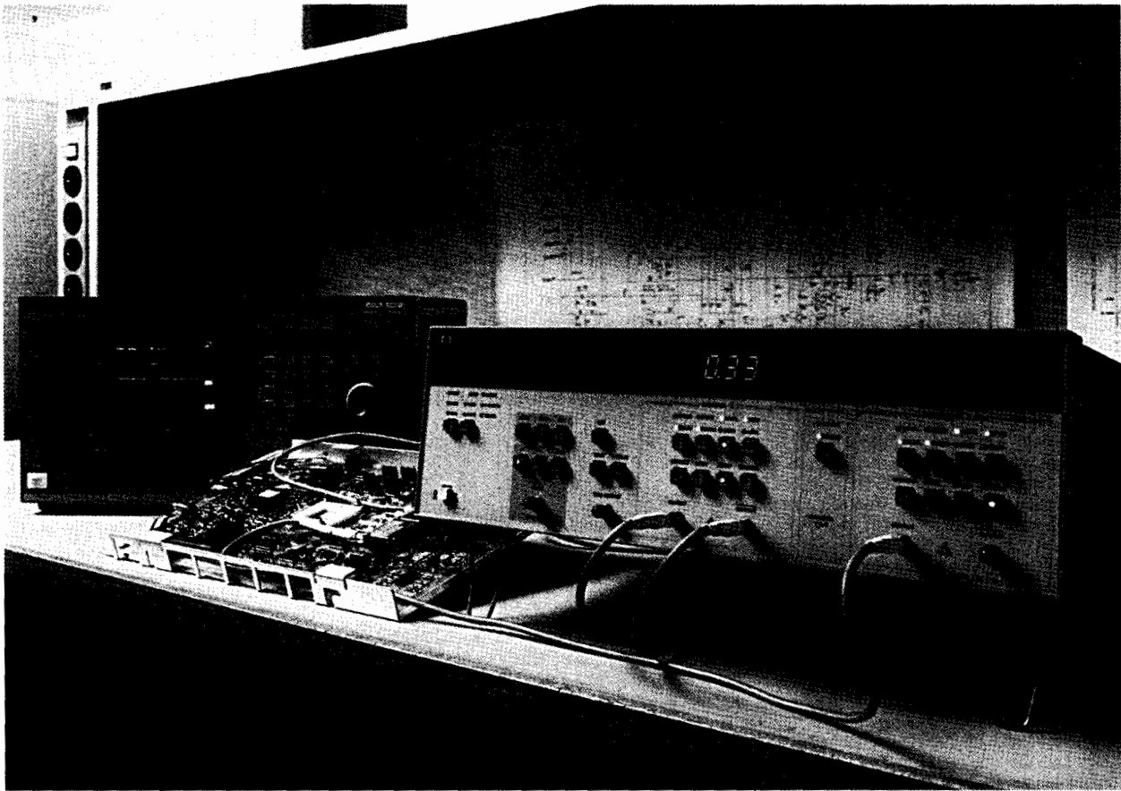
A typical stimulus-response test setup. The HP 8131A pulse generator in the foreground generates 500 MHz pulses with typically 120 ps transitions (20 to 80% of amplitude). The HP 54120 Series oscilloscope measures device response.
