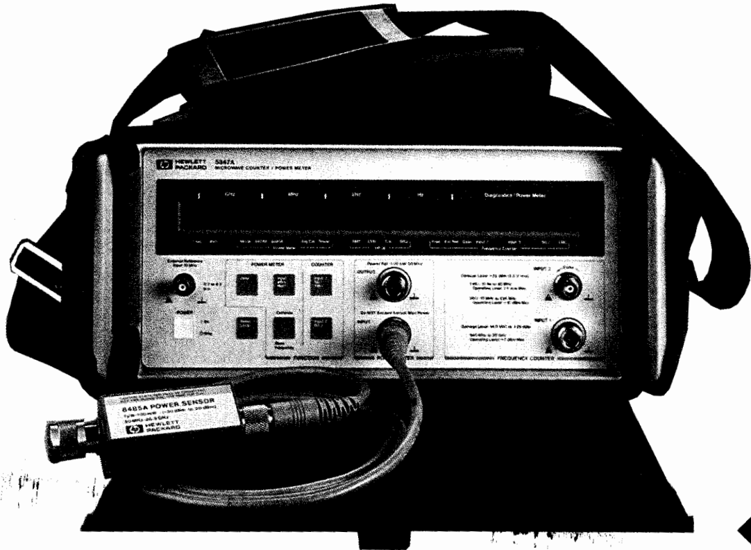
HP 5347A with optional soft carrying case and HP 8485A power sensor
